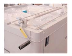
• Before dispensing, start winding the top of the liner into winder.
