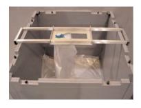
Install fill bridge across the top of the LiquiFold 315 and attach fill fitment to fill bridge.
