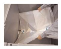
Attach grasping tool to glad adapter and place liner in container with dispense fitment end in first and lining it up with the bottom discharge of the LiquiFold 315. Hold the filling fitment up and bring to top of the container.
