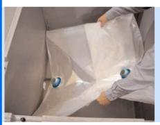
Attach grasping tool to glad adapter and place liner in container with dispense fitment end in first and lining it up with the bottom discharge of the LiquiFold 315. Hold the filling fitment up and bring to top of the container.
