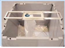
Install fill bridge across the top of the LiquiFold 315 and attach fill fitment to fill bridge.
